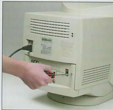
Fig 5 Opening a computer
