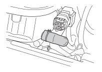
10.Remove the plug and drain water and oil at the periodic maintenance interval. The air cleaner drain plug is located beneath the air cleaner box.
