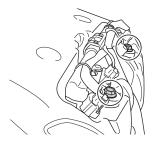
5. Remove the top feed injector bolts.
