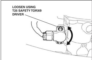
6. Verify TPS is set correctly. Verify the TPS operates in the following range:
