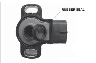
2. Using a T-25 safety Torx® bit, remove the upper and lower fastener for the primary TPS.
